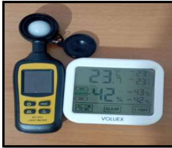
Image 04 showing light meter and thermo hygrometer that use it in climate study
